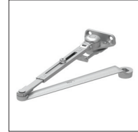
4020-3049FL Fusible link ■ Handed ■ Releases hold-open function, adjustable at shoe, when exposed to temperatures above 165° F ■ 3 7/8" (98 mm) maximum reveal ■ Optional ■ NOTE: Check local codes before specifying FL arms. NOT A life safety product!
